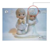
After you manually set the Slow Shutter Speed in the "Manual" capture mode, the shutter speed will be shown on the LCD screen when the shutter button is pressed halfway and the subject is focused.
